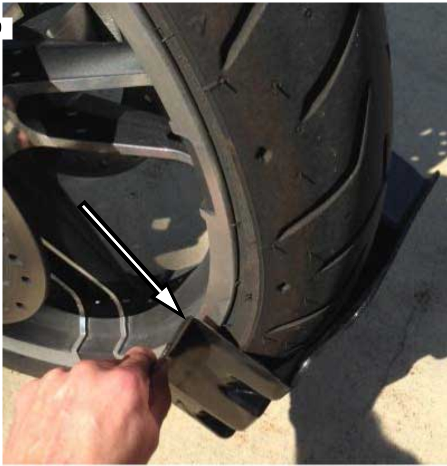
Figure 2. Removing Front Wheel Skid Spacer
