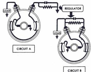
The same two circuits are used for insulated regulators except that a return wire is used between the regulator and generator instead of a ground return.
