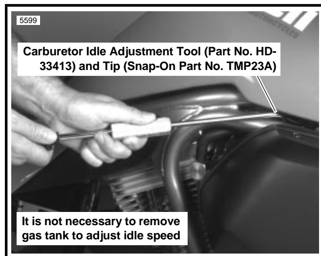
Figure 60. Adjusting Idle Speed
