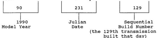
Transmission numbers are no longer hand stamped. Similar to crankcase numbers, they are "pin stamped" by machine. The numbers are block style and look as though they were formed by a series of "center-punched" dots.
