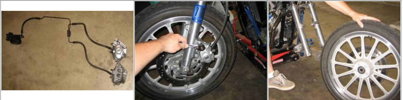
Installing the new rotors. Start all the bolts by hand then snug them up in a criss-cross pattern. Torque to spec (16-24 ft-lbs). 10)
