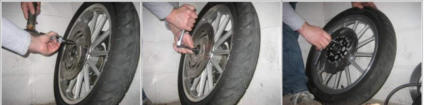
Installing the new rotors. Start all the bolts by hand then snug them up in a criss-cross pattern. Torque to spec (16-24 ft-lbs). 10)
