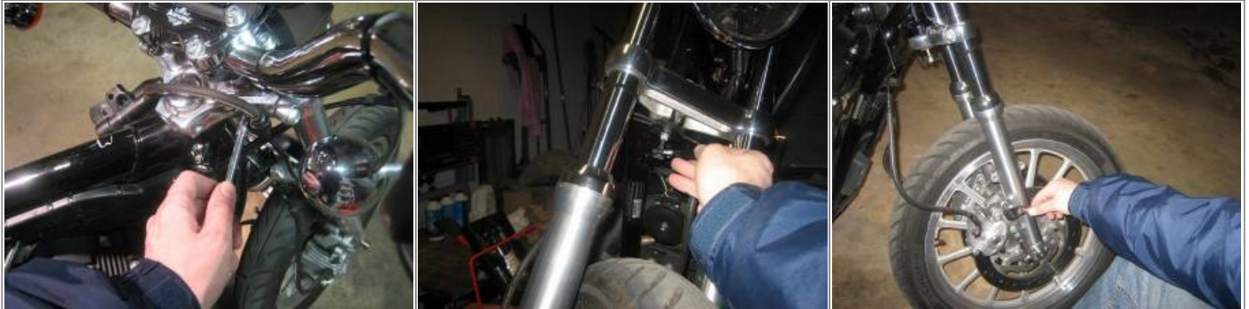
Brake line clamps removed from triple trees. A short bungee cord to hold the master cylinder out of the way to remove the calipers. 6)
