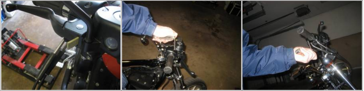
Brake line clamps removed from triple trees. A short bungee cord to hold the master cylinder out of the way to remove the calipers. 6)
