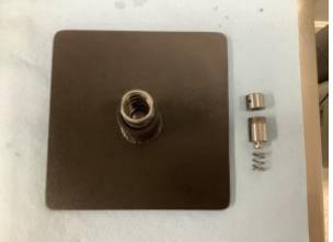
A doglegged pick works good for removing the retainer clip and removing the internals. A small flat head screwdriver works also.
