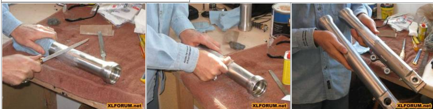
Filing the fender mounts off the fork sliders 3)
