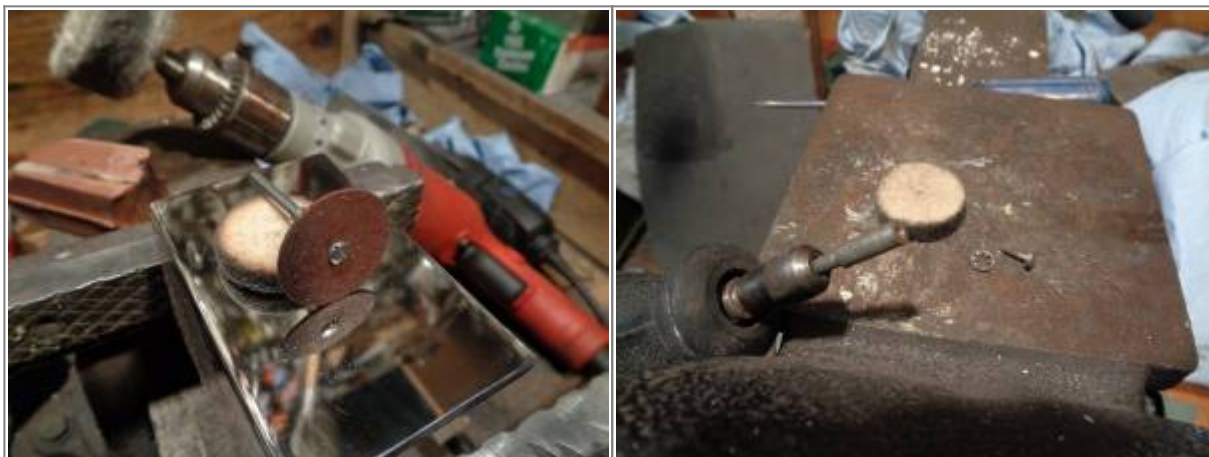
Dremil pad mounted to a cutting wheel mandrel 17)
