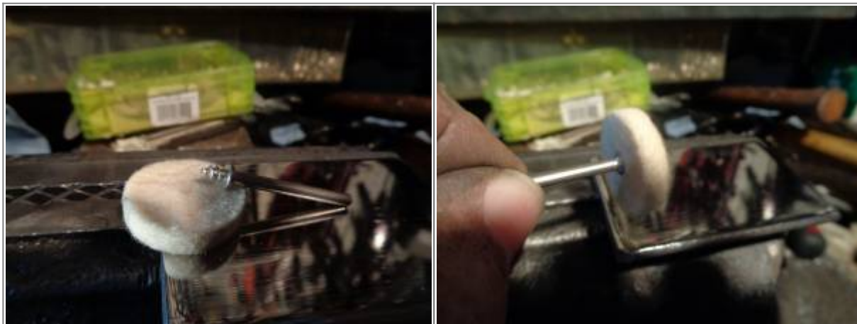
Dremil polishing pad mounted to a threaded shaft 16)
