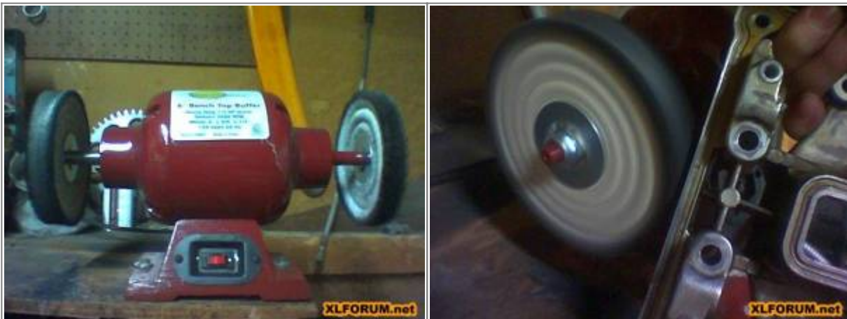
Polishing a rocker box top with a benchtop buffer 2) 3)
