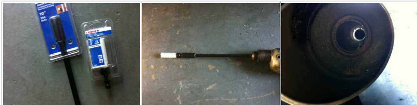
Drilling out exhaust baffle with a hole saw and extension. 7)
