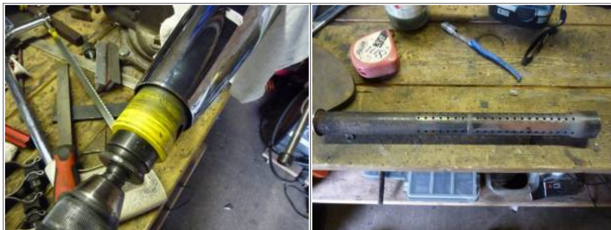
Removing an exhaust baffle with a hole saw. 8)
