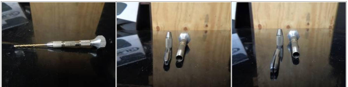
Testor hand held pin vise with a reversible collet for bigger drill bits 6)
