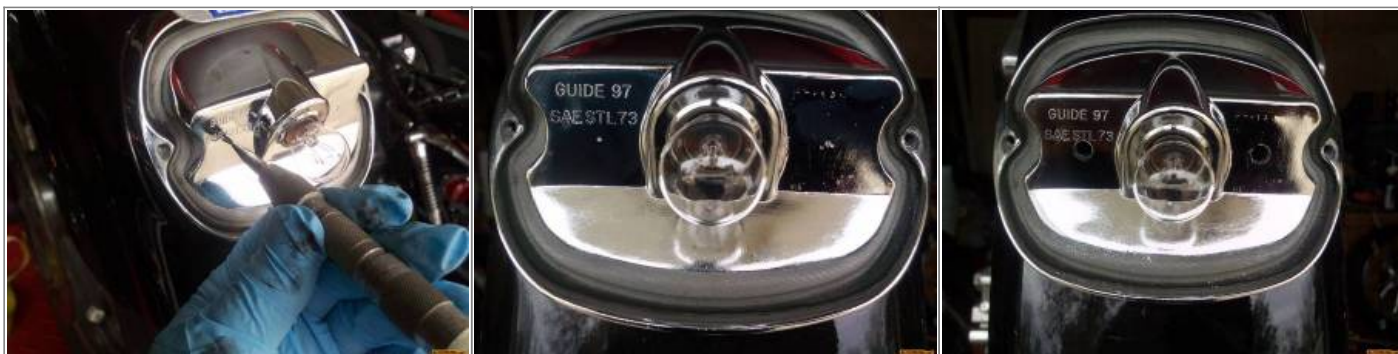
This punch was used to make a tail light mod for broken factory mounting studs 9)
