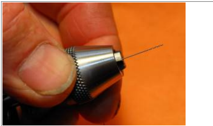
Pin vise made to fit into a regular drill chuck 4)
