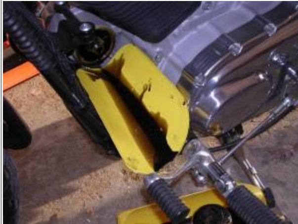
An old antifreeze jug with the side cut open making a drain pan and the cut piece is bent as a funnel. 21)
