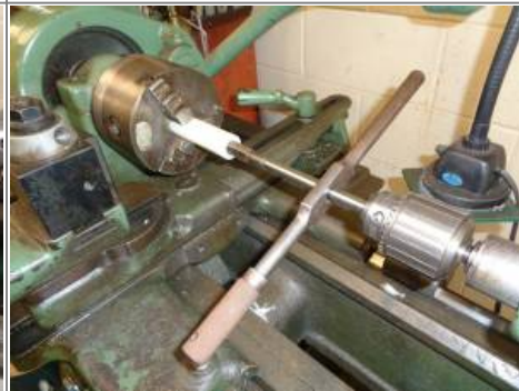
If made carefully, there is no need for a set screw on the nylon bushing. It's either the slip fit, chamfer on the inside rear of the hole from the drill bit, trapped air when the bushing is installed, composition of the nylon or a combination of these things that holds the bushing firm when pushed onto the pinion shaft. 21)
