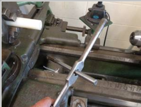
If made carefully, there is no need for a set screw on the nylon bushing. It's either the slip fit, chamfer on the inside rear of the hole from the drill bit, trapped air when the bushing is installed, composition of the nylon or a combination of these things that holds the bushing firm when pushed onto the pinion shaft. 21)
