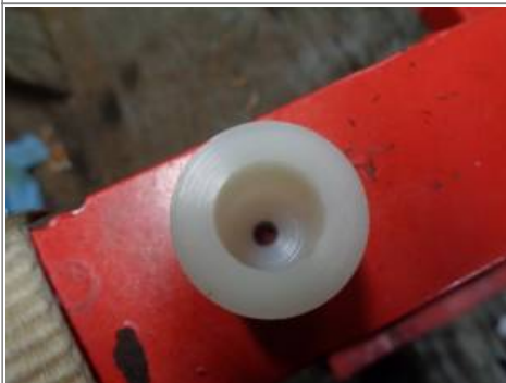
If made carefully, there is no need for a set screw on the nylon bushing. It's either the slip fit, chamfer on the inside rear of the hole from the drill bit, trapped air when the bushing is installed, composition of the nylon or a combination of these things that holds the bushing firm when pushed onto the pinion shaft. 21)
