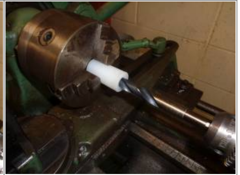
Bushing removed, cut to desired length and tapped for #10x32 threads. (same screw that holds the timing cup to #2 cam) 20)
