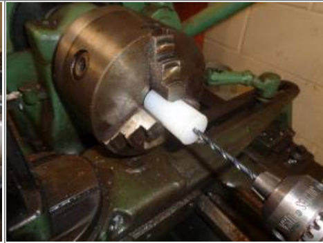
Reamer set in straight, "lightly" snugged into the chuck jaws enough to still spin by hand. Bushing is gently reamed by hand keeping down the heat. 19)
