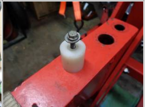
If made carefully, there is no need for a set screw on the nylon bushing. It's either the slip fit, chamfer on the inside rear of the hole from the drill bit, trapped air when the bushing is installed, composition of the nylon or a combination of these things that holds the bushing firm when pushed onto the pinion shaft. 21)
