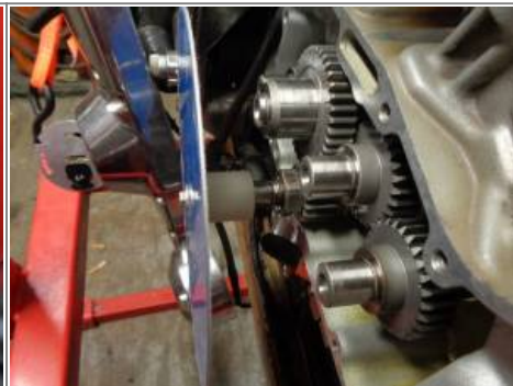
If made carefully, there is no need for a set screw on the nylon bushing. It's either the slip fit, chamfer on the inside rear of the hole from the drill bit, trapped air when the bushing is installed, composition of the nylon or a combination of these things that holds the bushing firm when pushed onto the pinion shaft. 21)
