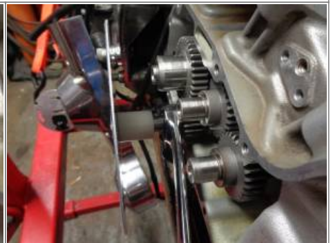
If made carefully, there is no need for a set screw on the nylon bushing. It's either the slip fit, chamfer on the inside rear of the hole from the drill bit, trapped air when the bushing is installed, composition of the nylon or a combination of these things that holds the bushing firm when pushed onto the pinion shaft. 21)
