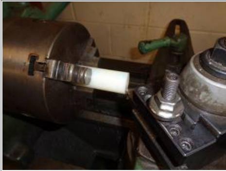
This tap wrench has a "V" slot in the tightening mechanism to allow for use with round tooling. 18)
