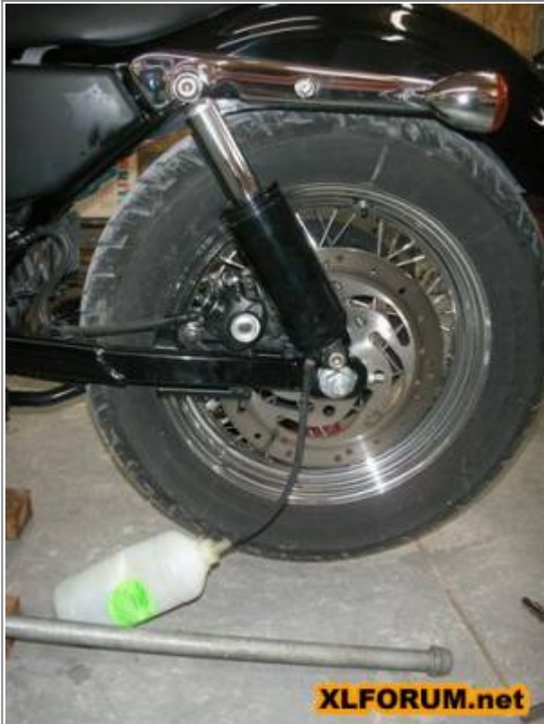
Removing RK shock oil 11)
