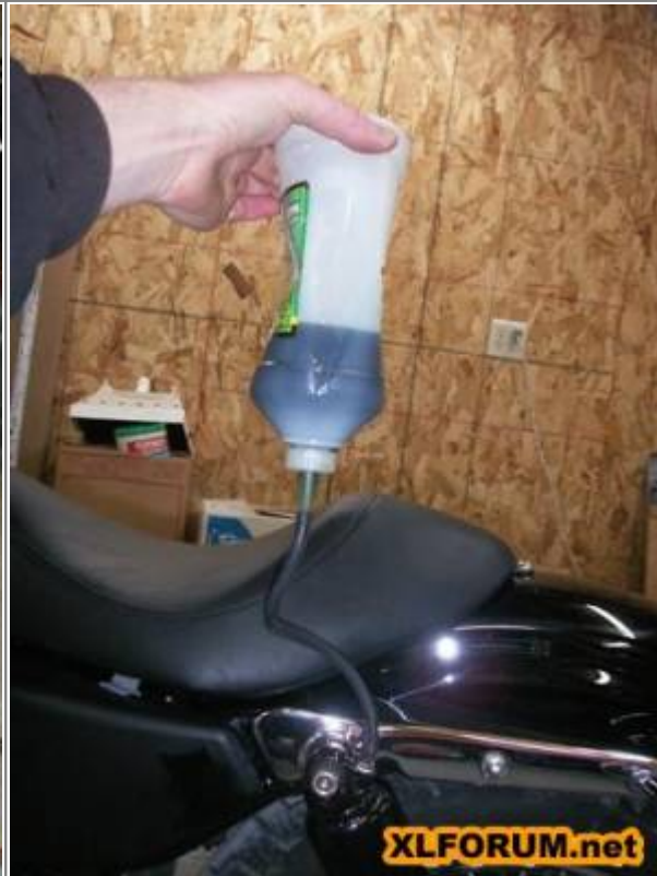
Installing RK shock oil 12)
