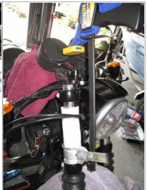
It may take a few goes to get it to depress squarely into the tube. Then just turn the socket until the threads on the cap start properly. 6)
