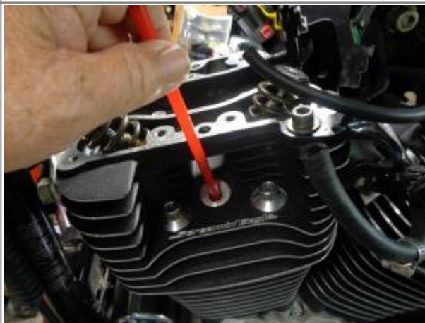
A straw in plug hole for finding TDC 1)
