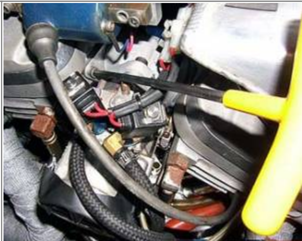
The easy way to get to the upper manifold bolts is to use a long T-handle ball end hex key wrench like this one from Bondhus
