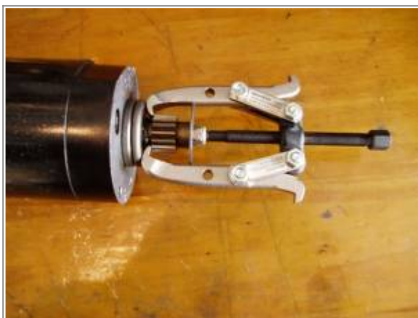
Two-jaw gear puller to pull the gear off the generator 2)
