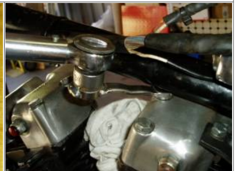
Torquing rear rocker box bolts with torque wrench extender. 4)
