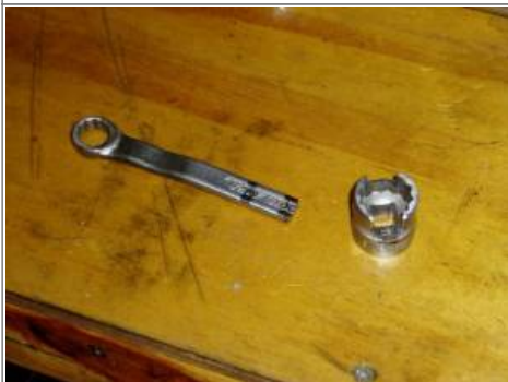
1/2" wrench cut down (box also ground down to fit confined areas) 3/4" socket notched with an angle grinder. 2)
