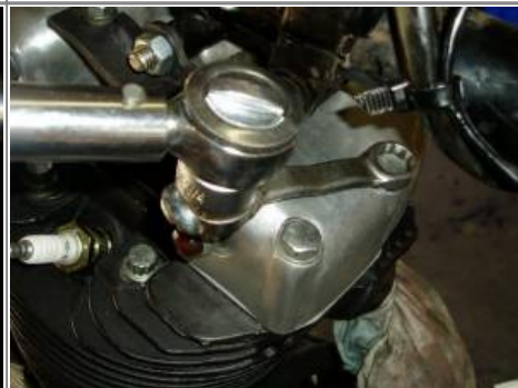
A little cutting, a little welding and you have a special wrench to reach the bolts under the frame. 5)
