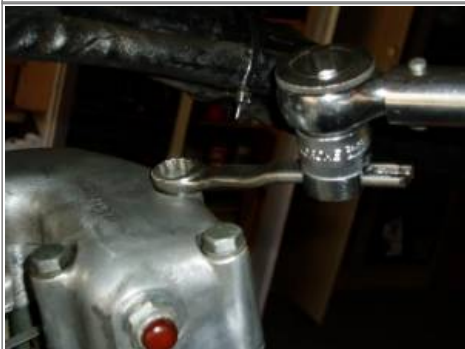
A little cutting, a little welding and you have a special wrench to reach the bolts under the frame. 5)
