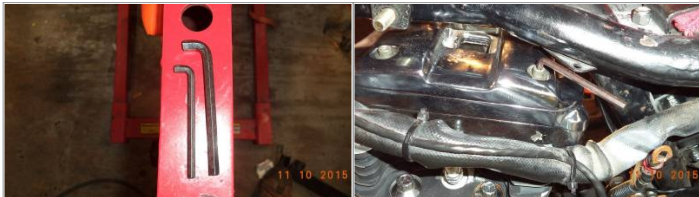
Allen wrench end cut shorter with a Dremil cut-off blade 7)
