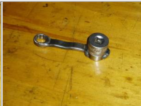
Torque wrench extender welded and ready to use. Extension Length: 3" from the center of the drive square to the center of the (intended) bolt. 3)
