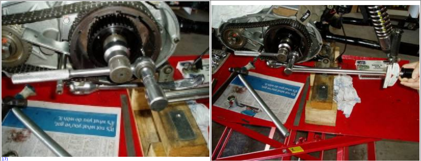
This application is used to adapt a 1/2" drive socket for use with a 3/4" drive torque wrench. Really! 18)
