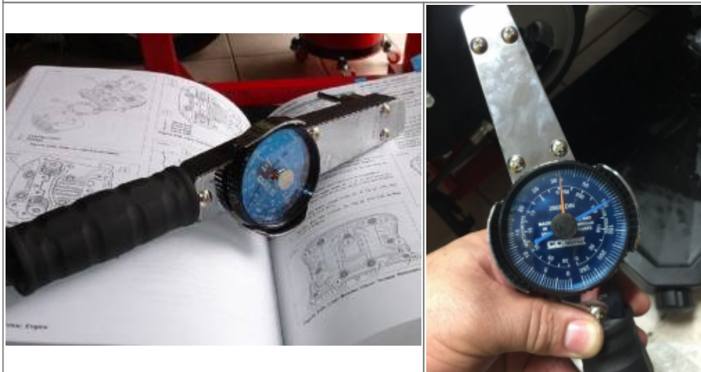
CDI (Snap-On) dial torque wrench. 3) 4) 0-250 in/lbs
