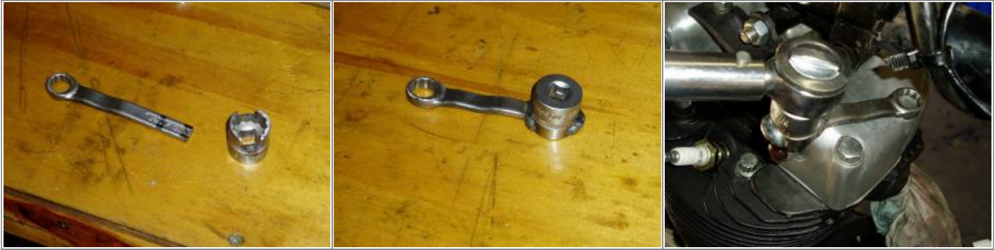
Homemade Wrench Extension for in-frame applications 15)
