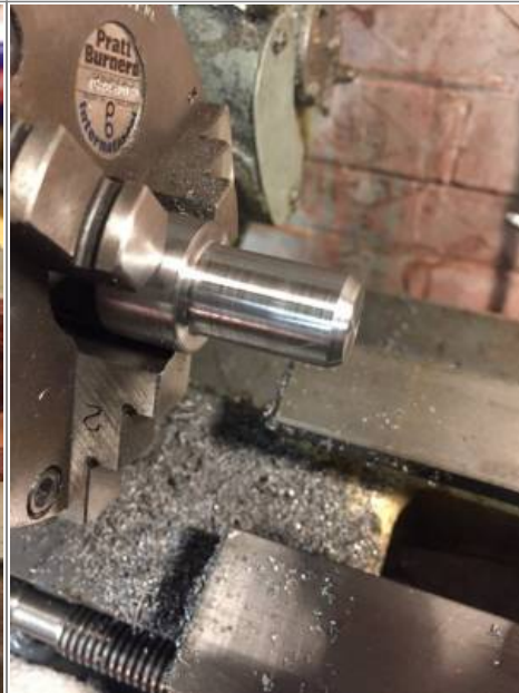
Cut a stepped bar in the lathe to fit the bearings. The big end got pressed into the socket. The step sits 3/16'' below the business end of the socket. 2)
