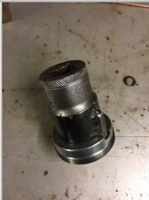
Cut a stepped bar in the lathe to fit the bearings. The big end got pressed into the socket. The step sits 3/16'' below the business end of the socket. 2)
