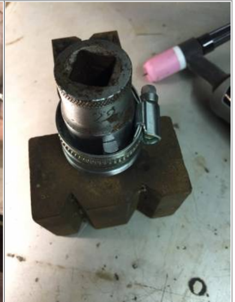
Held it together with a hose clamp for welding. 3)
