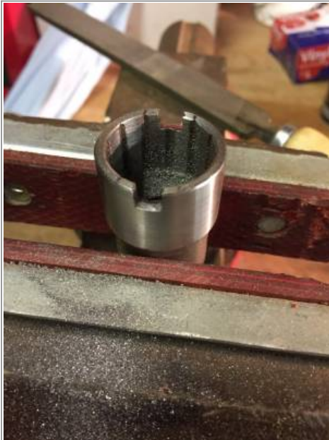
An old socket (ID larger than the sliding top hat spacer) with most of the teeth hogged. Cut some slots and made some little ears. 1)
