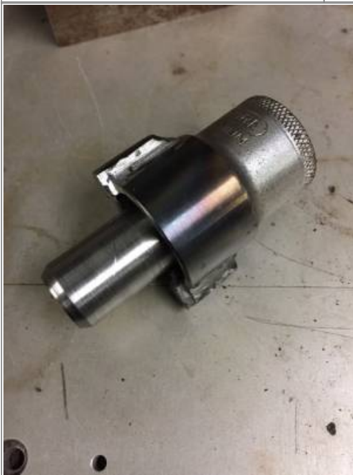
An old socket (ID larger than the sliding top hat spacer) with most of the teeth hogged. Cut some slots and made some little ears. 1)
