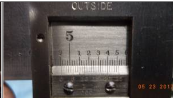
4.915" reading on a vernier caliper
