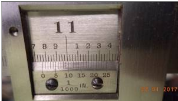
10.770" reading on a vernier caliper
