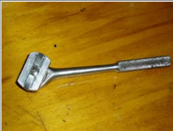
Commercially available primary filler plug tool used with a 3/8" socket wrench 2)
