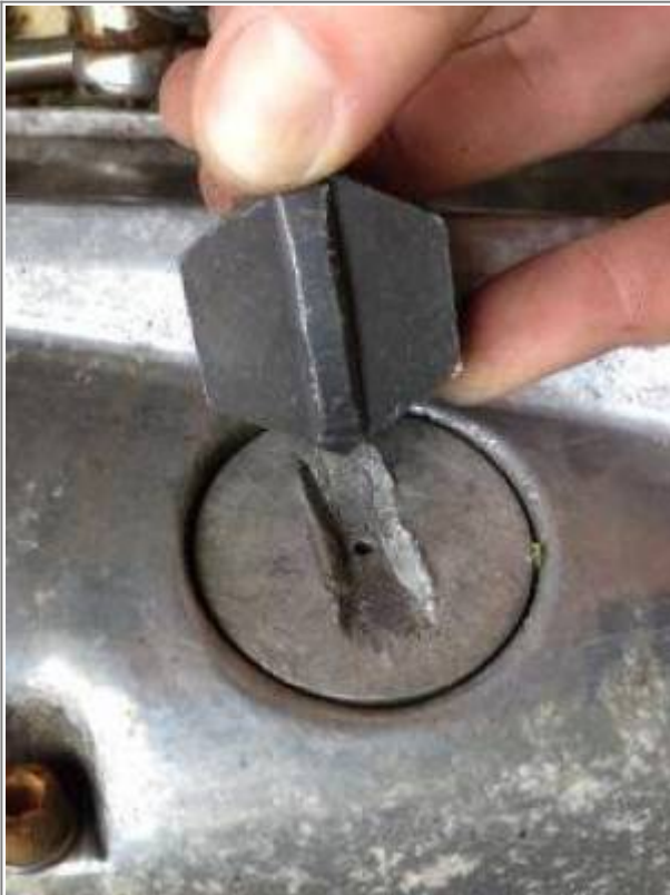
Sometimes, commercially available tools will not work due to previous over-torque or the wrong wrench used over time. 1)
