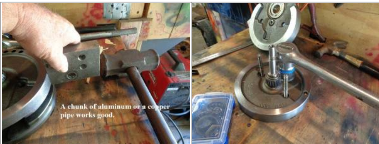
A block of aluminum and a sledge hammer works for knocking the flywheel loose.
