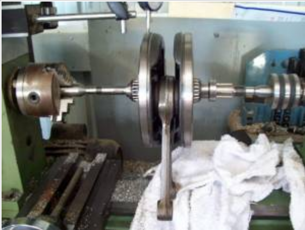
Truing flywheels on center in a lathe with no offset jigs 21)
