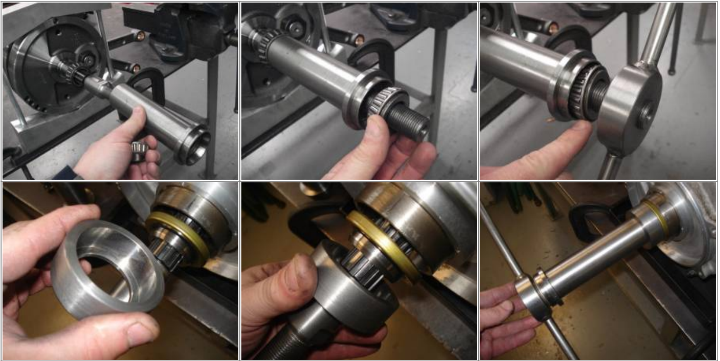
Homemade tool to pull the flywheels back into the left case, pressing the bearing on and pull the wheel in at the same time. 24)
