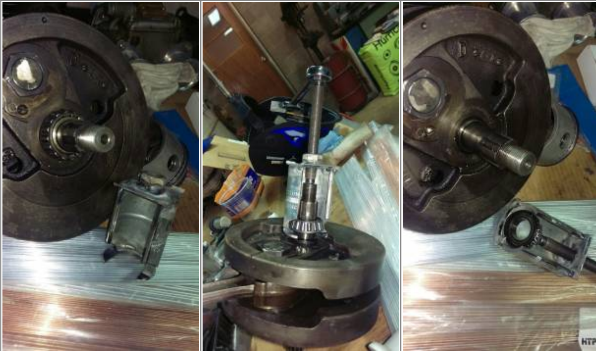
Homemade Timken Bearing Removal Tool 9)
