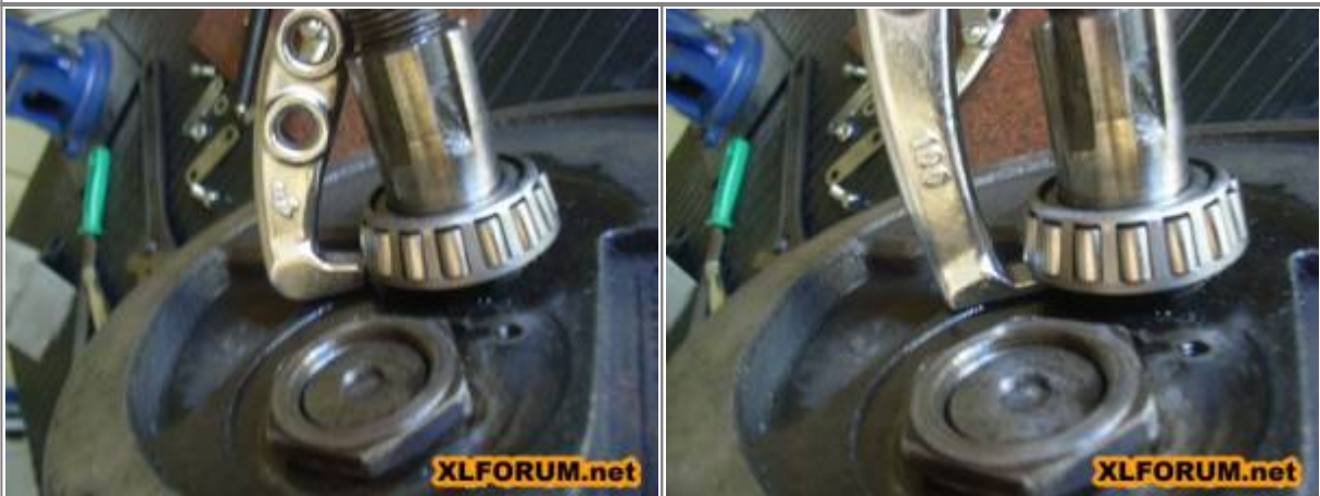
Gear Puller Mod for Removing Timken Bearings. (L)-before 9) , (R)-after 10)
