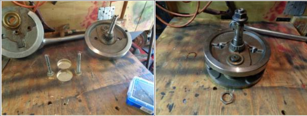
A block of aluminum and a sledge hammer works for knocking the flywheel loose.
