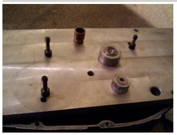
Then pull every thing apart. Make dowels and install. Open bolt holes in door where necessary. If you ever change to different door with different dowel size, pull old dowels and make stepped dowels.
