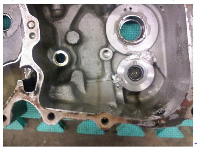
• Note that the welds are small enough that they can be removed to restore the original design. Some guys screw rings to the case with screws thru the .250 thick wall behind the ring instead of welding.
