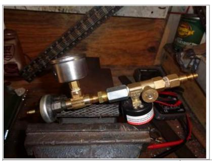
With zero pressure applied, the circuit is closed, continuity is achieved between the probes and the buzzer sounds off. 4)
