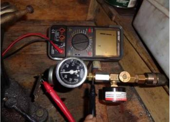
This switch didn't make contact until the pressure got down to about 2-1/2 PSI.
