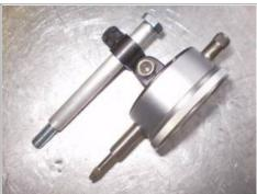
This is the dial indicator mounted on the alloy spacer
