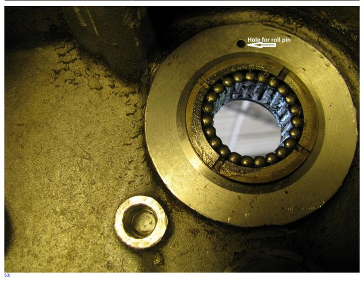
A roll pin is installed at the twelve o'clock position over the mainshaft hole to keep the spacers from spinning. The spacers on the end of the mainshaft have a tab that would hit the roll pin and lock in. If your mainshaft thrust washer has a tab, then it needs the roll pin. Otherwise it acts like an oil slinger, and them parts need that oil! Make sure to put the special hardened washer between the snap ring and the loose rollers.
