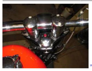
Wire up the +12 & oil pressure switch.
