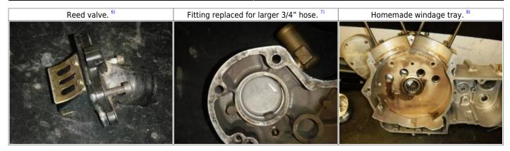
Cam box oil routing was also modified.
