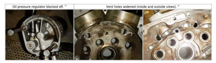
The umbrella valve in the cam cover was removed and a larger hose (3/4") fitting was added to use a reed valve for crankcase breathing instead.
