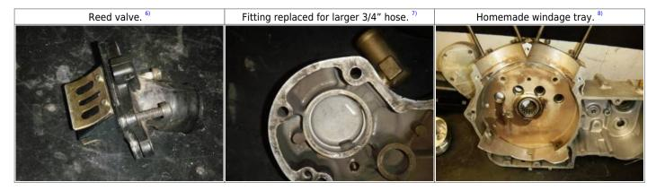
Cam box oil routing was also modified.
