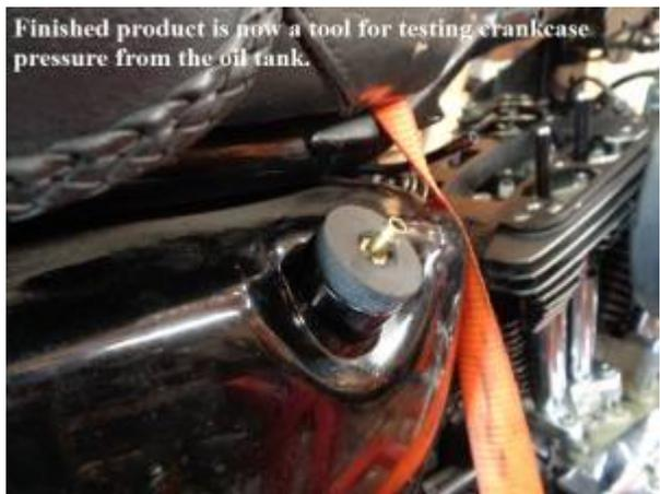
If you're testing the 04-up plastic oil tank for high pressure, the oil cap is not going to be helpful as a test point.
