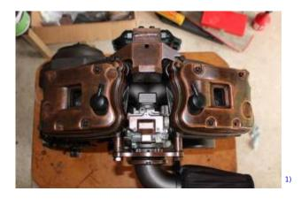
Some have reported better engine breathing and less oil leaking out the breather valve by using these Buell rocker boxes.
