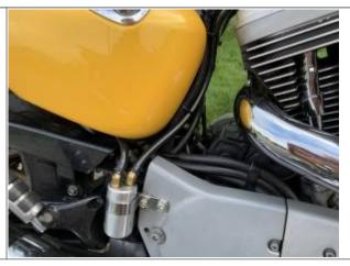
The tube from the catch can runs up under the fender and exits at the rear on the left side of the bike. When the bike is on the jiffy stand the hose is way over the side.
