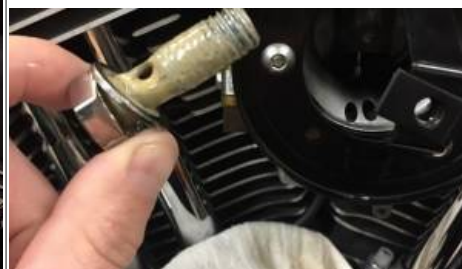
Rear bolt covered in sludge. 13)
