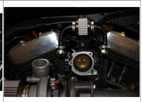
Filter mounted high will receive built up sludge. 14)
