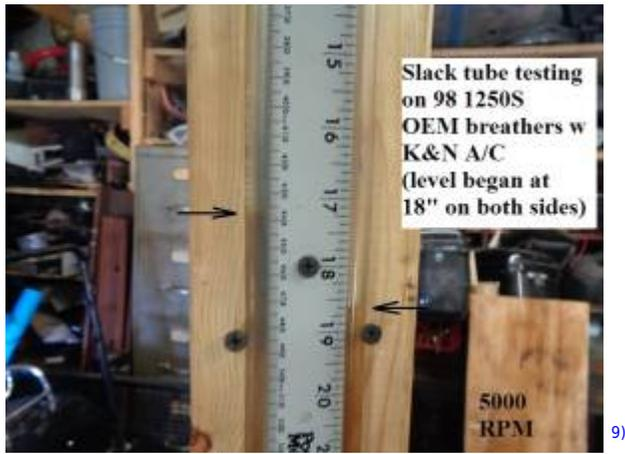
All future testing was done with the engine up to operating temperature with oil temp at 200°F.
