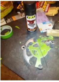
The VHT wrinkle plus went on gloss (very gloss) with at least 3 coats at varying angles and given a couple of hours for the paint to set.
