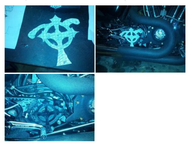
After settling on the pattern, it's just a matter of gluing on a paper pattern over the cover and cutting it out.
