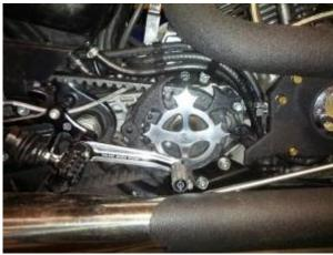
A brass woven mesh sheet was cut as a backing for the sprocket cover. (unpolished, mill finish, ASTM E2016-06, 12" width, 12" length, 0.025" wire diameter, 54% open area)
