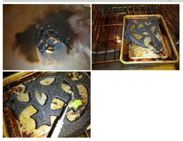
After it finishes curing, wash the adheasive off with solvent then block sand with 1000 grit wet to blend all lines back to crisp.
