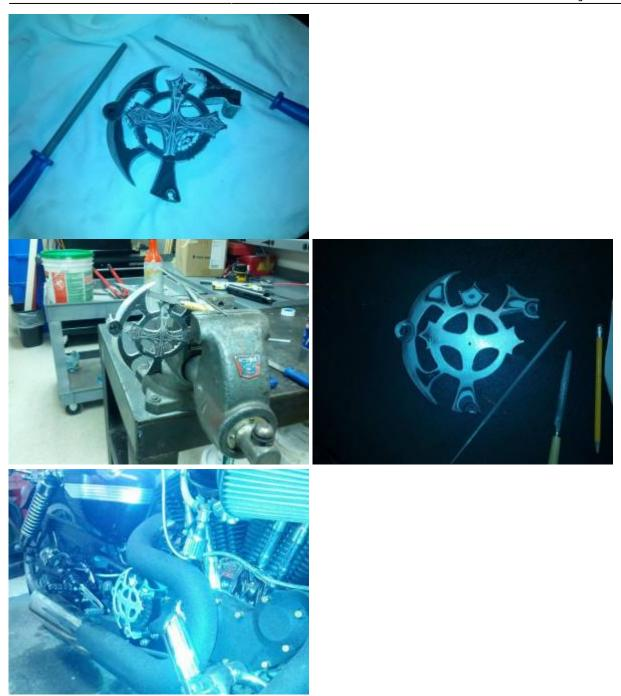
Finish shaping and sanded with sandpaper and getting ready for the wrinkle paint. The cross portioned was masked off to keep paint from sticking to it.
