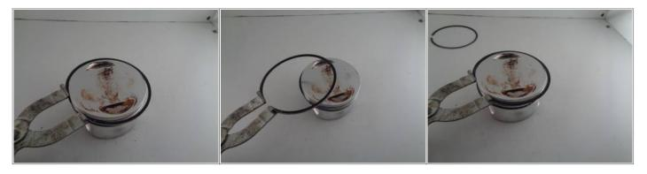
The oil rings are usually removed by hand.
