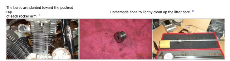
The hone was turned by hand for app. 10 turns (while holding the bushing in place) per lifter bore to clean up the scratches.
