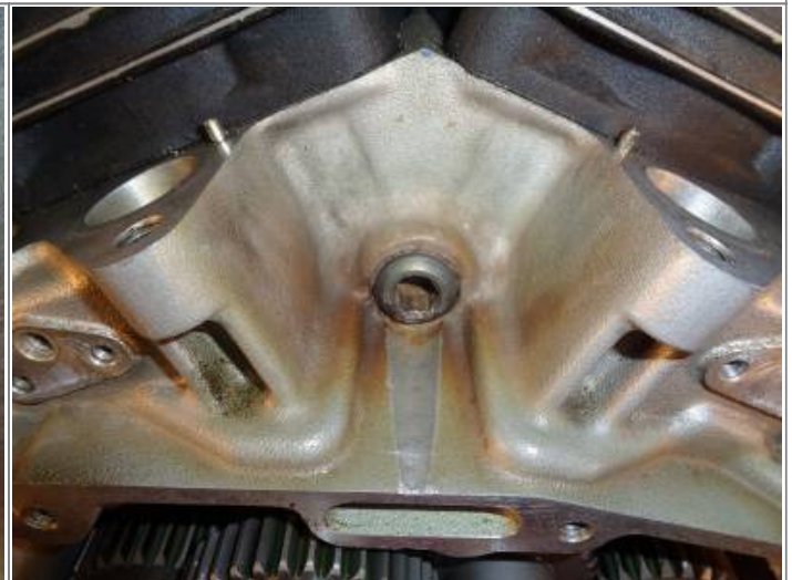
It's a good idea to chase the threads on the plug to match the newly refurbished threads in the case. Coat the threads with cutting oil and hand start the plug in the die to insure proper thread alignment
