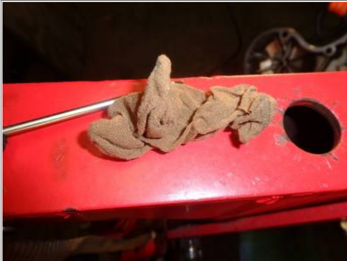
After chasing the threads. Notice the tap did not add any meat back to the threads. It simply straightens the threads (or what's left of them) back to their original condition. Install anti-seize on the plug threads and Teflon tape on the neck (if desired) and install the plug
