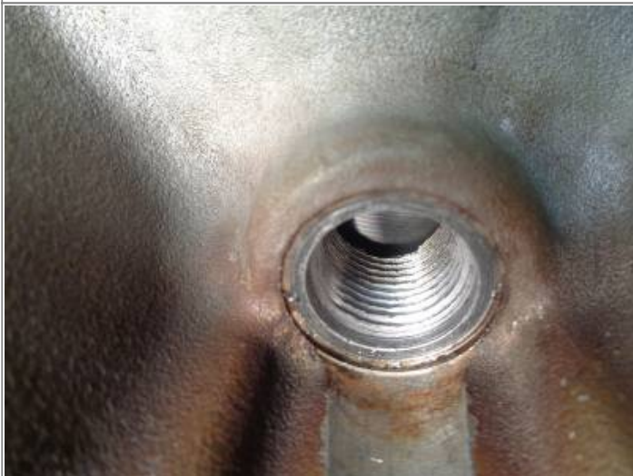
It's a good idea to chase the threads on the plug to match the newly refurbished threads in the case. Coat the threads with cutting oil and hand start the plug in the die to insure proper thread alignment
