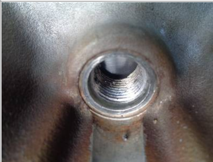
Remove the tap, clean it and repeat until your comfortable with the results
