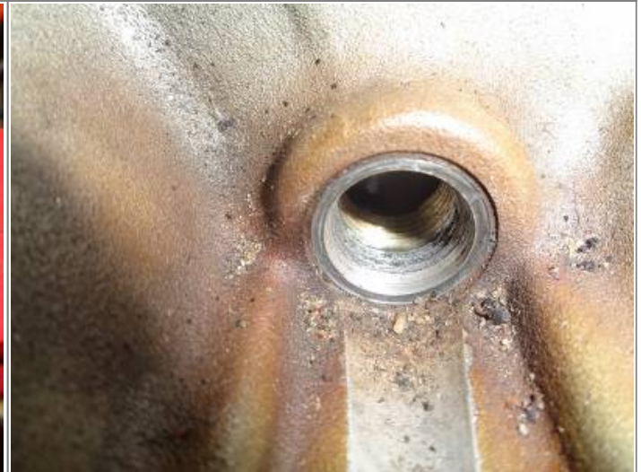
After chasing the threads. Notice the tap did not add any meat back to the threads. It simply straightens the threads (or what's left of them) back to their original condition. Install anti-seize on the plug threads and Teflon tape on the neck (if desired) and install the plug
