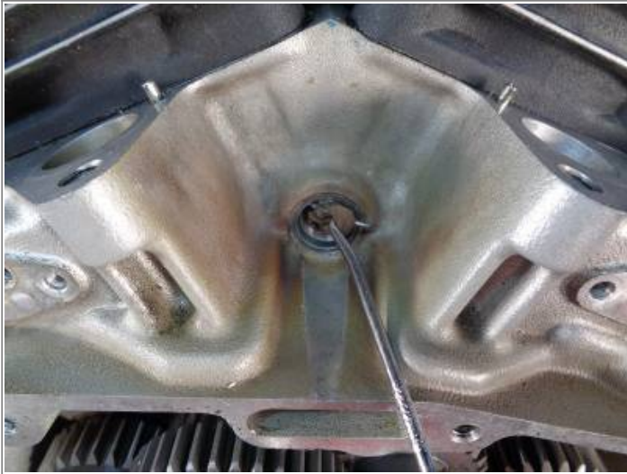
With the threads repaired, they now need to be cleaned up
