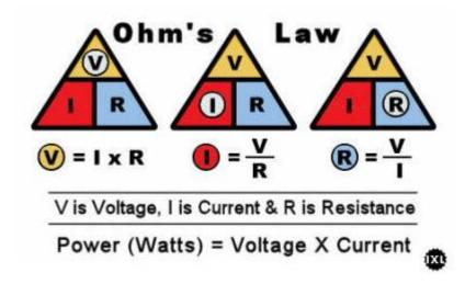
The above values for DC power are: Voltage in whole Volts, Current in whole Amps and Resistance in whole Ohms.
