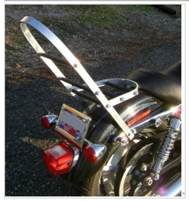
• Note the use of the small "L" bracket to secure the rack to the fender just behind the seat, using the available panhead bolt at said location and one additional through the front of the rack. I modified a piece of angle brace, drilling for the 1/4 x 20, shortening it to one hole in height, and rounding the ends on a grinder
