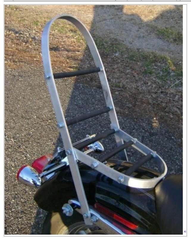
• The tour bags have been removed to allow a greater visual of construction. Had I wanted to run with-out bags, I would have ground the ends of the sissy bar more round
