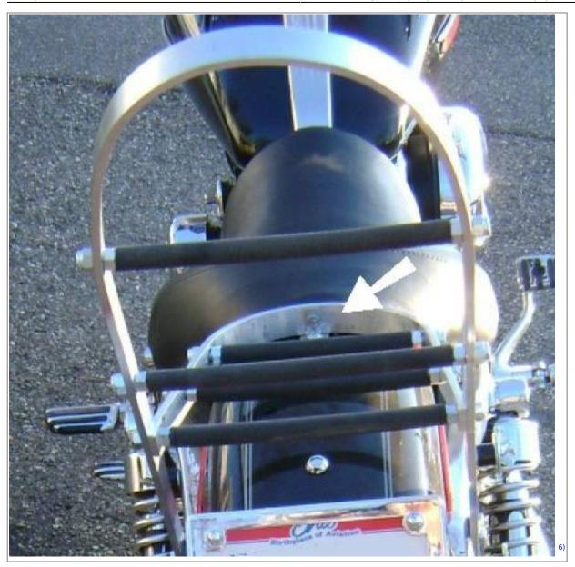
• The sissy bar is secured with a 5/16" bolt through the existing hole in the fender and fender bracket, having already moved the turn-signals to a rear mount. Note that additional strength is given to the bar by using the second hole as a "stop" bolt with 5 washers acting as a 1/4" spacer. This insures the sissy bar from pivoting backwards and pulling loose the bolt atop the fender
