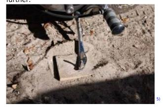
The kits want you to drill near the shaft/foot of the Jiffy Stand. If you try to attach from there with a Hugger the stand will not completely retract.
