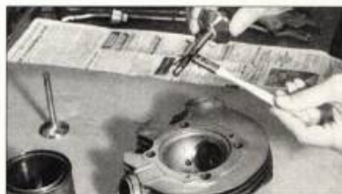
Next, lubricate the valve stem with a good assembly oil and place it in its guide.
