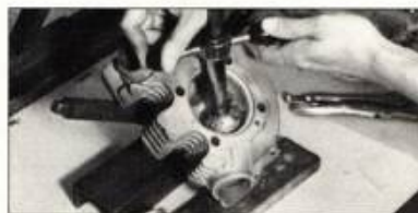
Valve seats are cut with a piloted cutter set. There are three different cutters; one for each angle of a standard three-angle valve job.
