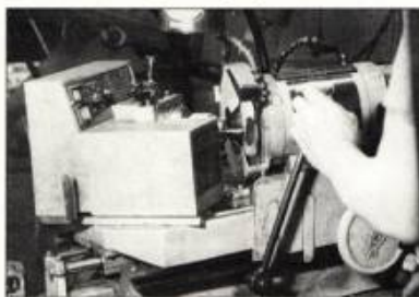
Even a new valve should be lightly faced just to be sure.
