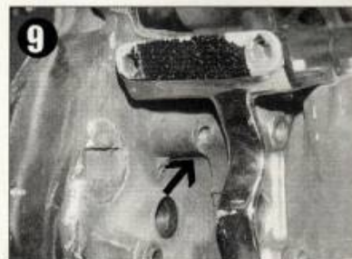
Be sure to check the rest of the case for cracks, too. This missing chunk (see arrow) should be replaced — by welding — but can easily be overlooked during a pre-purchase inspection.
