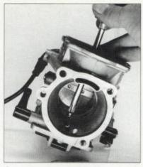
6 Don't lose the small silver section of the emulsion tube that we're pointing to with the screwdriver. It must remain in place to be used with the Thunderslide emulsion tube.
