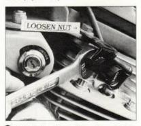
2 Installation is much easier with the carb off the bike. When loosening the big steel nut behind the choke nut bracket, remember to turn the nut clockwise, or the plastic threads will be destroyed.
