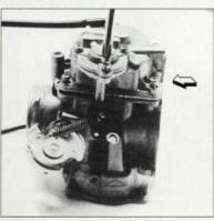
screws at the corners of the float bowl (see arrow). Do not remove the screws we're taking out unless you want to inspect the guts of the accelerator pump.
