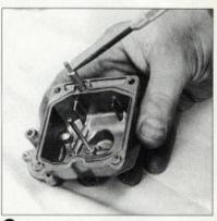
Locate the accelerator pump nozzle on the edge of the float bowl (we are pointing to it). Remove the bowl gasket.
