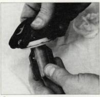
Carefully pull the rubber diaphragm off the stock slide. Make sure you remember which is the "up" side of the diaphragm. Install the diaphragm onto the Thunderslide kit's black plastic slide, sandwiching it between the snap-on plastic washers.
