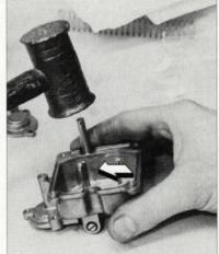
Drop the Thunderslide check ball and spring into the enlarged hole. Align the Thunderslide nozzle so the squirt hole faces the brass tube in the center of the bowl (see arrow). Tap nozzle lightly into place using a soft or brass hammer.
