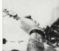
Measure the float level and make sure it is correct. Read your service manual for how to do this and the required specifications.
