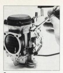
8 Remove the four screws on top of the carb and the big screw on the cable guide in order to remove the carb's top, spring, and slide.
