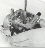
Install the Thunderslide emulsion 7 tube. Select a main jet (the instructions are very helpful about how to do that) and screw it into the emulsion tube.
