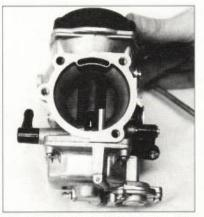
The Thunderslide's black plastic slide and big accelerator pump nozzle are plainly visible on this assembled CV. After you've reinstalled the carb on your Sportster, you're ready to start kickin' butt and takin' names.
