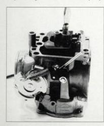
S Remove the float bowl, then remove the stock main jet and brass emulsion tube. Sometimes they come out together.
