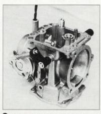
8 Using the supplied drill bit, carefully pierce the aluminum plug covering the idle mix screw. Remove the pierced plug with the supplied screw.
