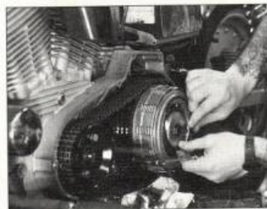
4 Rich carefully compresses the diaphragm spring with the correct tool and removes the snap ring that allows the pressure plate to be removed.
