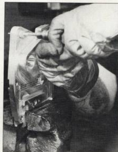
16 Rich lightly hones the dowel-pin holes in the new door so it will fit snugly, without being hammered into place. The fit is correct when you can lightly tap the door onto the dowel pins.
