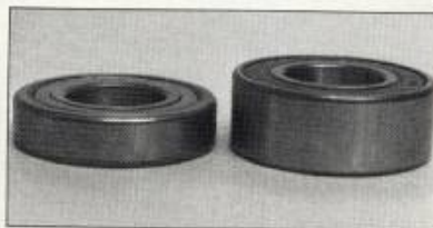
13 The bearing on the left is the stock door bearing. The bearing on the right is the double-row bearing from Zipper's.
