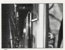
Look parallel to the disc towards the caliper to see the friction material against the disc inside the caliper. (A flashlight will help out a lot.) The distance from the disc to the metal that the material is bonded to must be at least 1/16" or the pads should be replaced.
