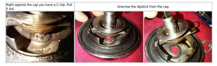
There is an O-ring at the top of the shaft between the cap and the wing nut. If it's flattened, it may cause an oil leak on the top of my tank.
