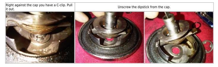
There is an O-ring at the top of the shaft between the cap and the wing nut. If it's flattened, it may cause an oil leak on the top of my tank.
