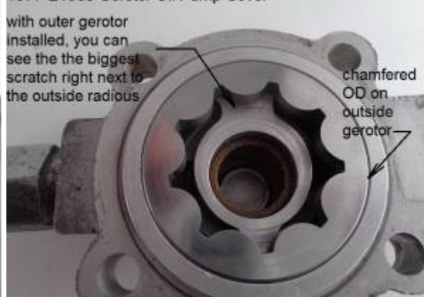
1977-E1983 Gerotor Oil Pump Cover
