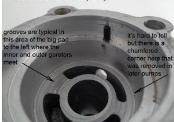
1977-E1983 Gerotor Oil Pump Body
