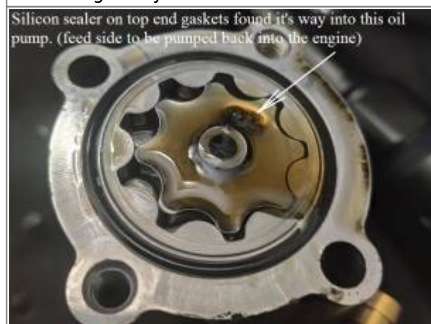
Silicone 'gummy bear' sheet found in the feed side 2)
