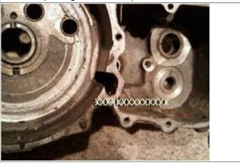
• So oil flowing unchecked into the pump from the oil supply line leaks clear thru engine into primary before it can start to fill the cam chest.
