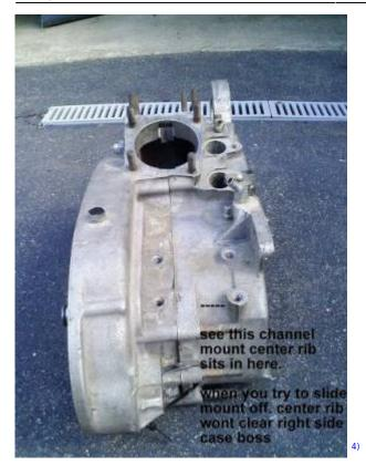
Examples of ways to cut the rear mount off without splitting the cases for a Pingel replacement mount.
