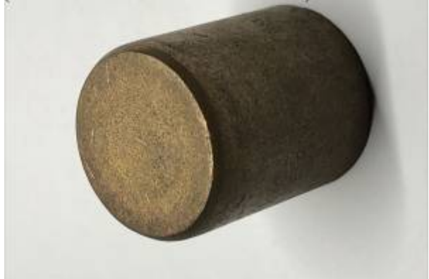
1975-1976 Sportster Shifter Shaft Bushing 34037-75 (closed on one end and resides in the cam cover)
