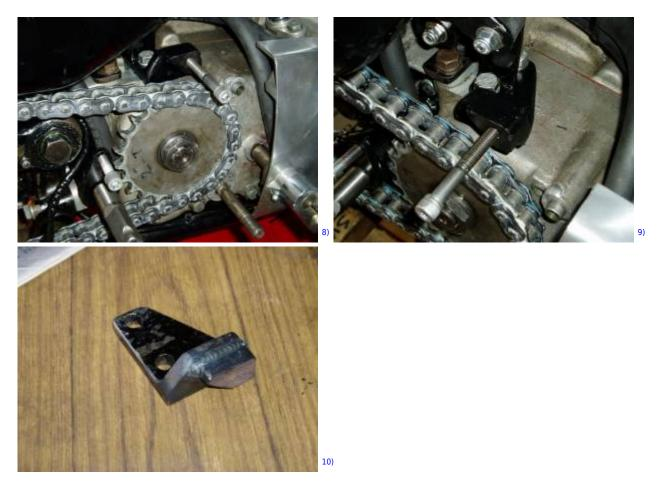
I shaped and had welded a piece of a 3/8" aluminium plate inside the sprocket cover.
