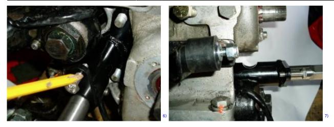
And here is the factory support bracket fix kit in place around the kick starter shaft.
